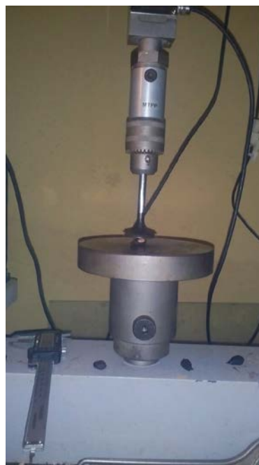
Figure 1: A gmelina seed undergoing compressive loading
